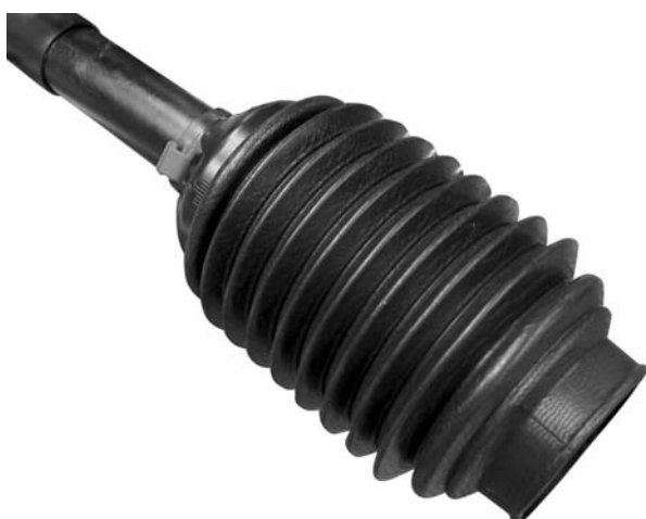
Figure 3.3 : Protection de la transmission
